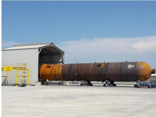
None of the two ← process separators made for the Eni refinery in Sannazzaro
